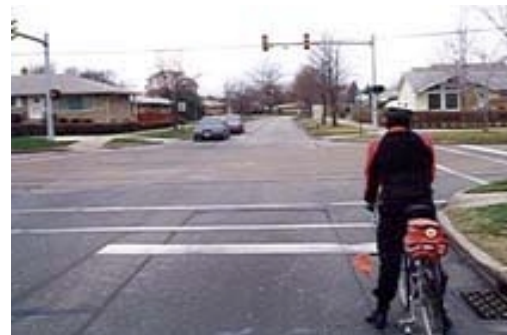
Simple Loop Detector: Detector wires are under the cyclist's left foot and another near left side of lane. (He should be further left.)
